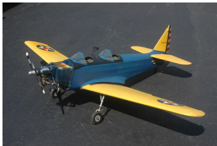
P-19, 80" WS. Powered by OS/120. Color matching cowl Nelson glow driver
