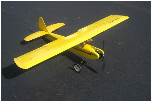
SR Batteries Cutie. 46" ED, geared brushless, 4 channel. A fun plane to fly. I may keep it.
