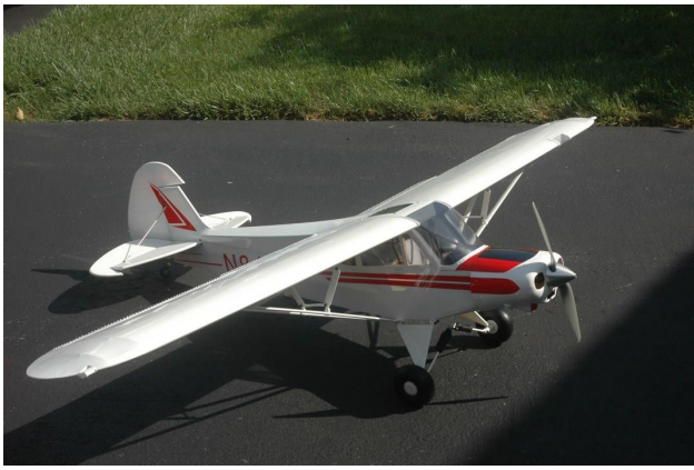
Electifly Super Cub. 68" electric. Flown only for MAN review. 5 channel, inc. flaps. Uses 4S 3200 mAh LiPos
