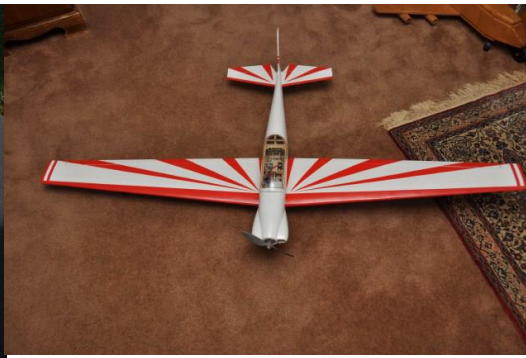
Model of Fournier RD-4, I think. Motor glider, 4 channel, perhaps 50" ws. Out runner. Needs 3S1600 LiPo
